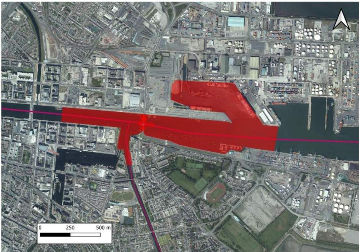
**Figure 9** *Local 2-D model with 1=D reaches defining flow and elevation boundary hydrographs at west (Liffey Estuary, south Dodder Estuary and east Dublin Port reach)*
