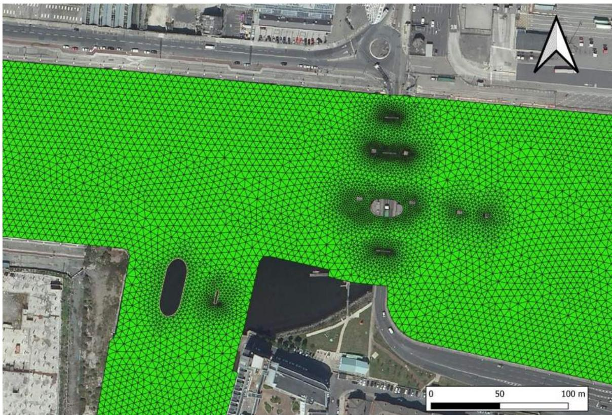
Figure 11 View of Telemac2D mesh structure – proposed case
