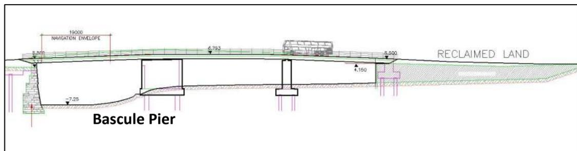
**Figure 2** Cross Section of Upstream face of Bridge
