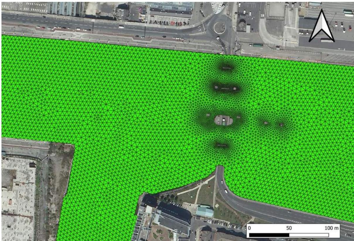
Figure 10 View of Telemac2D mesh structure – existing case.
